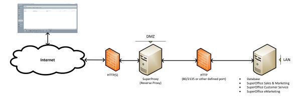
This may be the case when installing the SuperOffice modules; Customer Centre and SuperOffice eMarketing. These modules need to be available for external users to be able to "interact" with the CRM database. In these cases some traffic need to be routed from the internet to your domain and using the described Proxy server. The latter should be sufficient for any network administrator in terms of keeping security in place. The reverse proxy solution is used by most of the ASP providers today.
